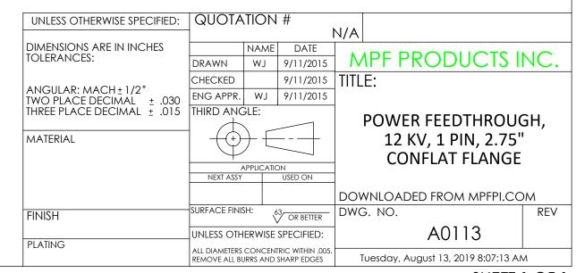
Power Feedthrough, 12 KV, 1 Pin, 0.250" Conductor, 2.75" Conlat Flange, UHV Rated, Bakeable to 450°C
