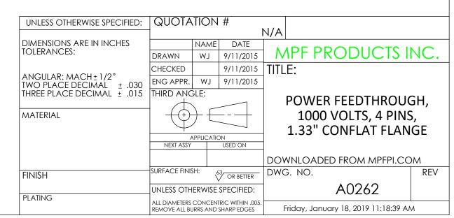
Power Feedthrough, 1000 Volts, 4 Pins, 0.050" Conductors, 1.33" Conflat Flange, UHV Rated, Bakeable to 450°C
