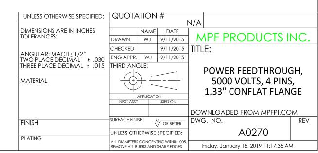
Power Feedthrough, 5000 Volts, 4 Pins, 0.050" Conductor, 1.33" Conflat Flange, UHV Rated, Bakeable to 450°C
