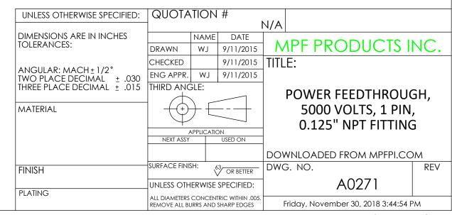
Power Feedthrough, 5000 Volts, 1 Pin, 0.125" NPT Fitting, UHV Rated, Bakeable to 450°C
