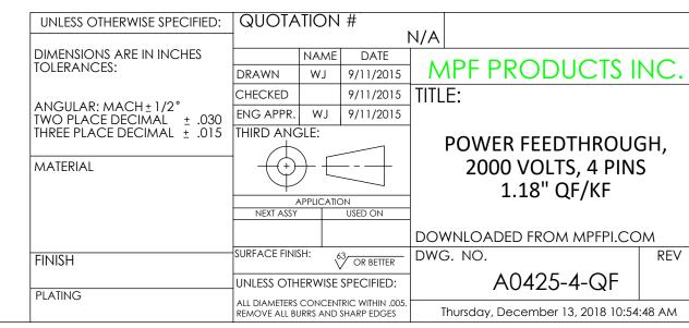
Power Feedthrough, 2000 Volts, 4 Pins, 0.056" Alumel Conductors, 1.18" QF/KF, UHV Rated, Bakeable to 450°C
