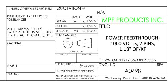
Power Feedthrough, 1000 Volts, 2 Pins, 0.050" Conductor, 1.18" QF/KF, UHV Rated, Bakeable to 450°C
