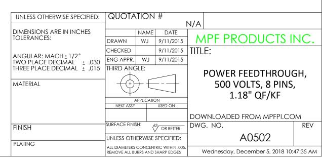
Power Feedthrough, 500 Volts, 8 Pins, 0..032" Conductor, 1.18" QF/KF, UHV Rated, Bakeable to 450°C
