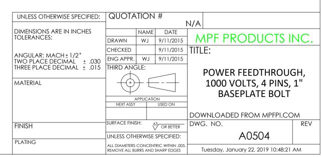
Power Feedthrough, 1000 Volts, 4 Pins, 0.050" Conductor, 1" Baseplate Bolt, UHV Rated, Bakeable to 450°C
