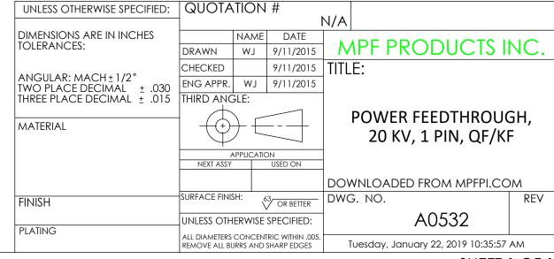
Power Feedthrough, 20 KV, 1 Pin, 0.092" Nickel Conductor, QF/KF, UHV Rated, Bakeable to 450°C
