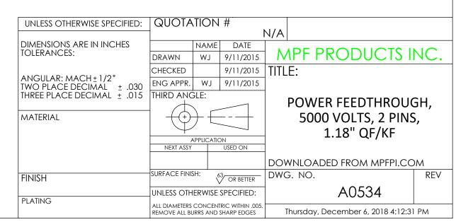
Power Feedthrough, 5000 Volts, 2 Pins, 0.050" Conductor, 1.18" QF/KF, UHV Rated, Bakeable to 450°C
