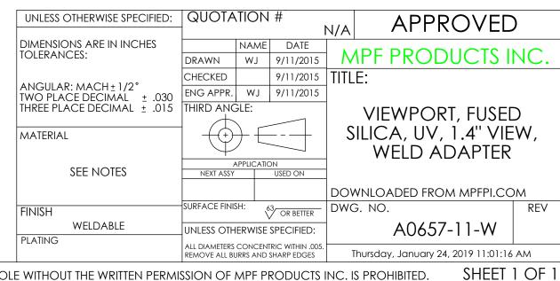
UV Grade Fused Silica Viewport, 1.37" View Dia, 1.50" Dia Stainless Steel Weld Adapter
