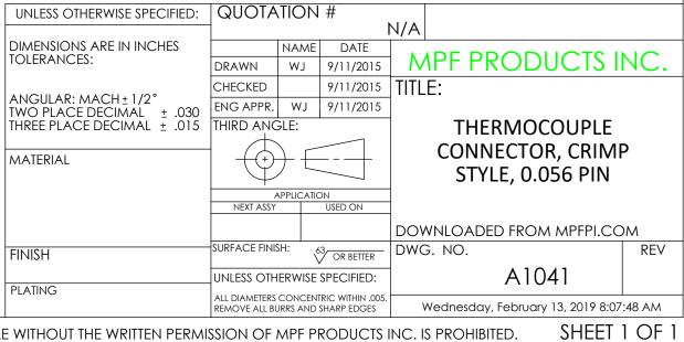
Push-on Thermocouple Connector, 0.056" Dia Pin, Package of 5
