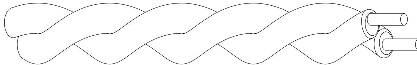
Kapton Insulated In-Vacuum Wire, Solid Core, Thermocouple Pair (Twisted), Type-K, 30 AWG, 96" length
