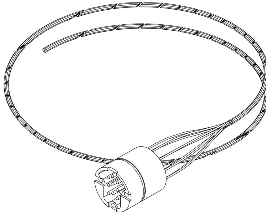
THE CABLE JACKET IS A PEEK BRAID WITH A NOMINAL DIAMETER OF 0.14 INCHES.
