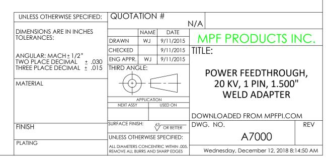
Power Feedthrough, 20K V, 1 Pin, .250" Conductor, 1.500" Dia. Stainless Steel Weld Adapter, UHV Rated, Bakeable to 450°C
