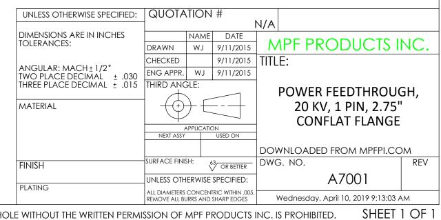
Power Feedthrough, 20K V, 1 Pin, .250" Conductor, 2.75" Conflat Flange, UHV Rated, Bakeable to 450°C
