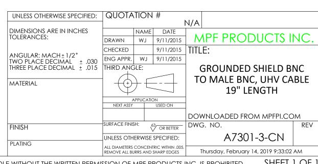
Coaxial Cable Assembly, In-Vacuum, Grounded Shield BNC to Male BNC, 50 Ohm Coaxial Cable w/ Kapton Insulation, 19" Length
