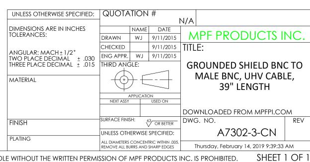
Coaxial Cable Assembly, In-Vacuum, Grounded Shield BNC to Male BNC, 50 Ohm Coaxial Cable w/ Kapton Insulation, 39" Length
