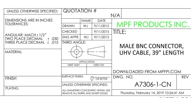
Coaxial Cable Assembly, In-Vacuum, Male BNC to Cable, 50 Ohm Coaxial Cable w/ Kapton Insulation, 39" Length
