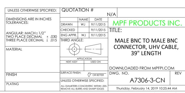
Coaxial Cable Assembly, In-Vacuum, Male BNC to Male BNC, 50 Ohm Coaxial Cable w/ Kapton Insulation, 39" Length
