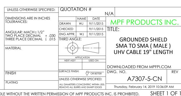
Coaxial Cable Assembly, In-Vacuum, Grounded Shield SMA to SMA (Male), 50 Ohm Coaxial Cable w/ Kapton Insulation, 19" Length
