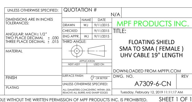
Coaxial Cable Assembly, In-Vacuum, Floating Shield SMA to SMA (Female), 50 Ohm Coaxial Cable w/Kapton Insulation, 19" Length
