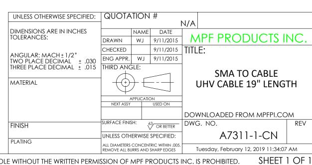
Coaxial Cable Assembly, In-Vacuum, SMA to Cable, 50 Ohm Coaxial Cable w/ Kapton Insulation, 19" Length
