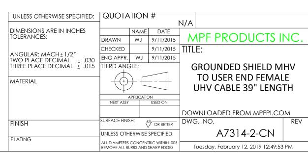
Coaxial Cable Assembly, In-Vacuum, Grounded Shield MHV to User End Female, 50 Ohm Coaxial Cable w/ Kapton Insulation, 39" Length
