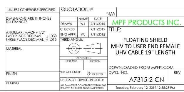
Coaxial Cable Assembly, In-Vacuum, Floating Shield MHV to User End Female, 50 Ohm Coaxial Cable w/ Kapton Insulation, 19" Length
