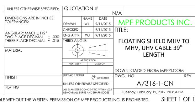
Coaxial Cable Assembly, In-Vacuum, Floating Shield MHV to MHV, 50 Ohm Coaxial Cable w/ Kapton Insulation, 39" Length
