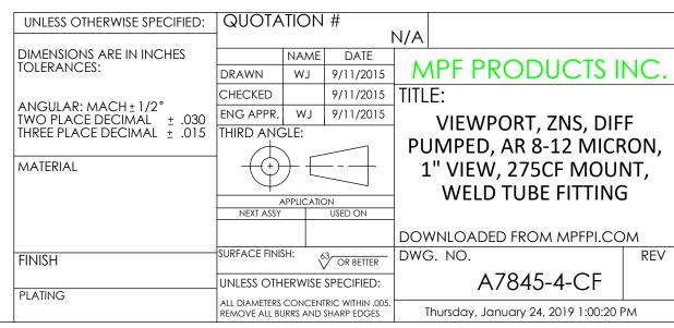
Cleartran (ZnS) Viewport w/ AR Coating for 8-12 microns, Differentially Pumped, 0.90" View Dia, 2.75" Conflat Flange, Weld Tube Fitting
