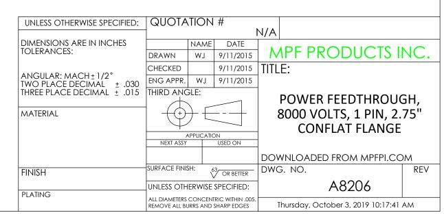
Power Feedthrough, 8000 Volts, 1 Pin, 0.500" Conductor, 2.75" Conflat Flange, UHV Rated, Bakeable to 450°C
