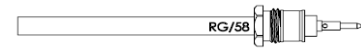
STEP 4: SOLDER PIN TO CONDUCTOR MAKING SURE NOT TO OVERHEAT AND MELT THE PLASTIC SPACER.
