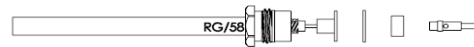
STEP 3: MOVE LOCKING BOLT, REGULAR WASHER, AND GROMMET TOWARD STRIPPED END OF CABLE, THEN PUSH METAL SPACER INTO THE GROMMET AND BRAID (BRAID SHOULD BE BETWEEN THE METAL SPACER AND GROMMET) FOLLOWED BY THE THIN WASHER AGAINST THE METAL SPACER, PUSH PLASTIC SPACER AROUND THE DIELECTRIC WITH THE LARGER DIAMETER STEP TOWARD THE THIN WASHER AND PUSH THE PIN ONTO THE CONDUCTOR MAKING SURE IT IS INSERTED INTO THE PLASTIC SPACER.
