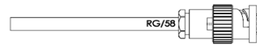
STEP 5: INSERT CABLE SUB ASSEMBLY INTO THE HOUSING. HOLD CABLE AND BODY IN PLACE AND TIGHTEN THE LOCKING NUT WITH A WRENCH.
