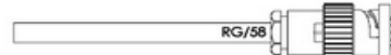
STEP 5: INSERT CABLE SUB ASSEMBLY INTO THE HOUSING, HOLD CABLE AND BODY IN PLACE AND TIGHTEN THE LOCKING NUT WITH A WRENCH.
