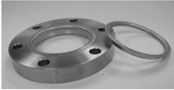
Figure 2. High-temperature weld-in window cell. The cell is shown both before welding, and welded into a test flange. The weld collar and flange are titanium, and the window material is sapphire. Included with permission of MPF products, incooperated 1 .
