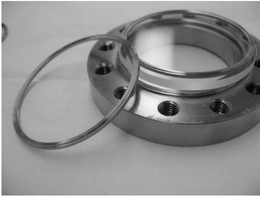
Figure 6. Picture of a sapphire window with knife edge gaskets resting on a vacuum flange. These parts are those shown in Fig. 5 with the exception of the window cap. There is a third copper gasket leaning against the whole assembly.
