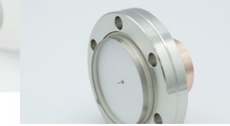
Broadband transmission of RF signals into cryogenic UHV Cavity. 50 Ohm Impedance Matched. Copper-alloy components sealed to alumina ceramic. UHV metal-sealed flange mount. Integrated liquid cooling.
