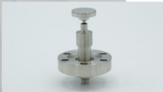
LEReC CAD Beam Position Monitor with 30mm button antenna.
