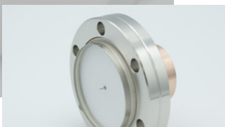
Broadband transmission of RF signals into cryogenic UHV Cavity. 50 Ohm Impedance Matched. Copper-alloy components sealed to alumina ceramic. UHV metal-sealed flange mount. Integrated liquid cooling.
